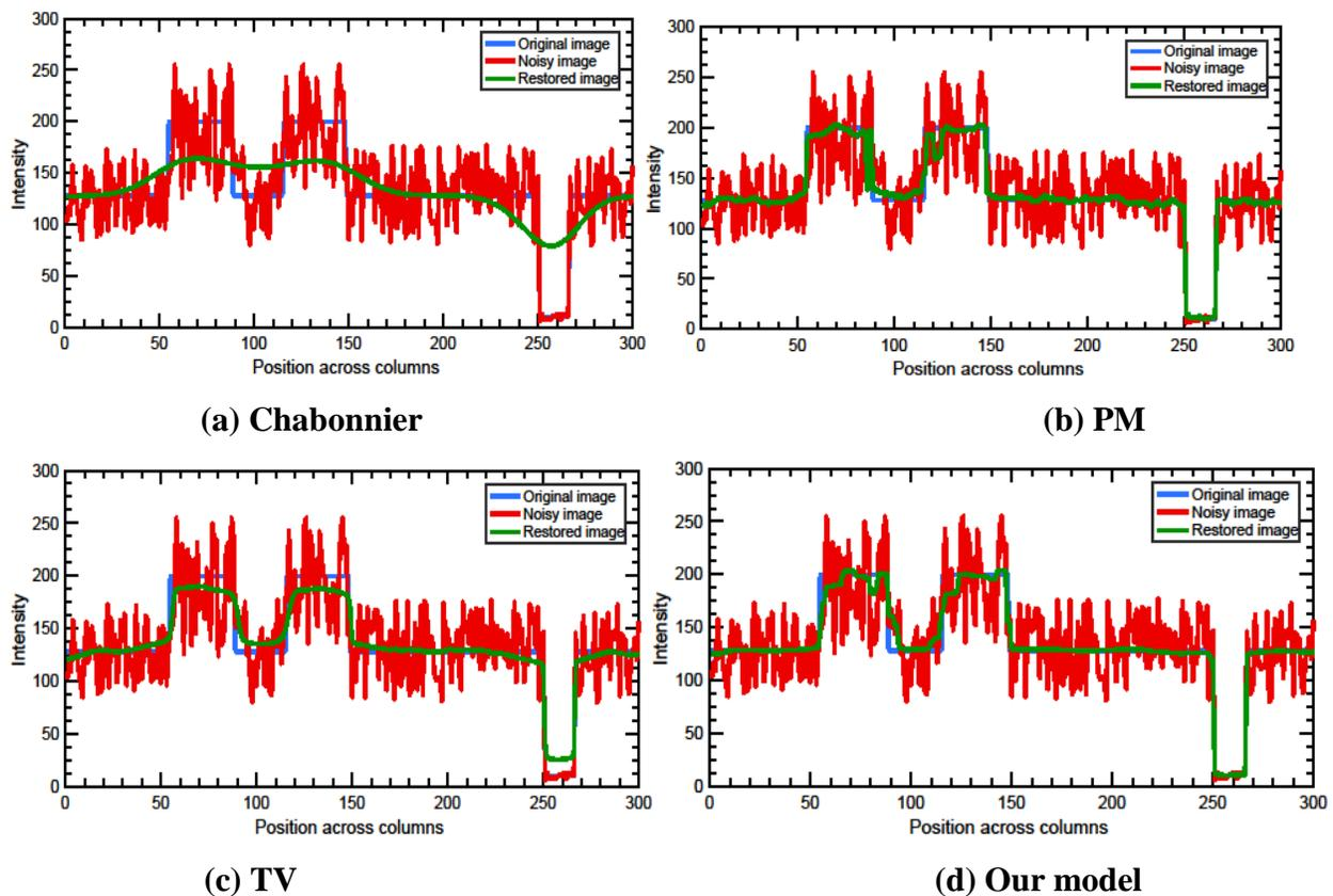
Figure 4: Intensity image profiles of different denoising methods.
