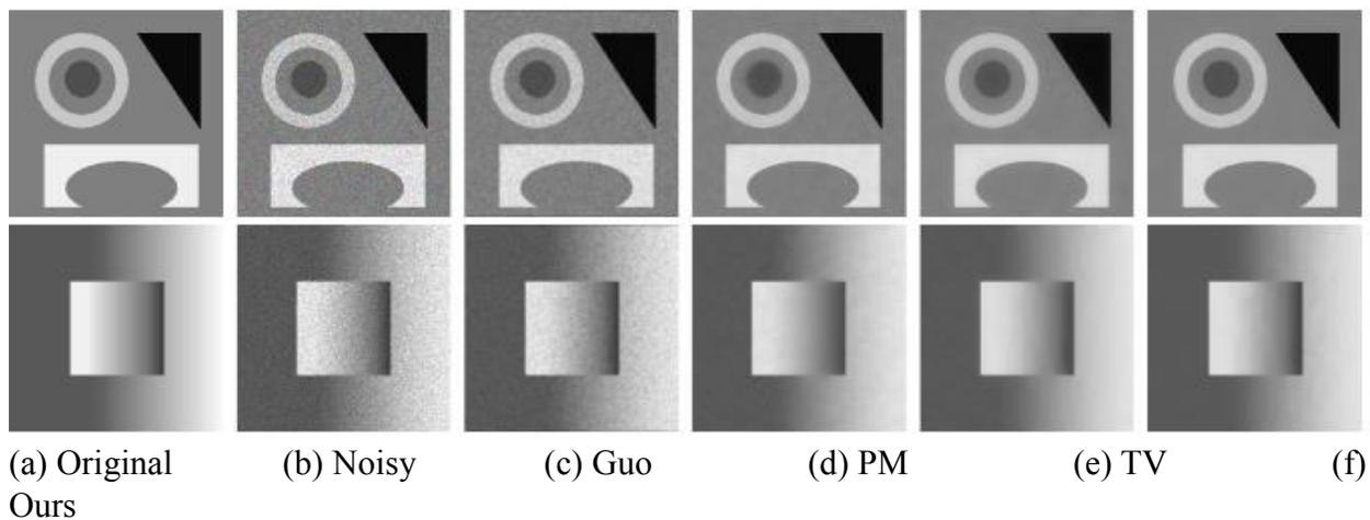
*Figure 5: Different denoising methods applied on the noisy synthetic images: first row, denoising results of “Geometry”; and second row, “Squares” synthetic images. PM (Perona-Malik) and TV (Total Variation).*
