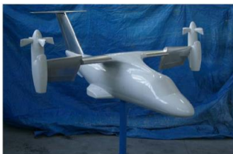
Figure 6: Windform Tunnel Final Model (1:8 scale) for the Prototype of the Tilt Rotor ( www.additivemanufacturing.com , 2014).
