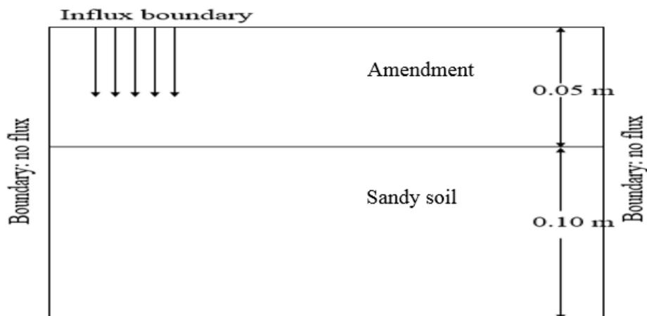
*Figure 2: 2D geometry of soil column model*
