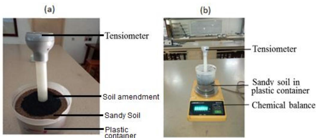
Figure 4: Photographic images of the laboratory experimental unit showing (a) soil amendment application (band method) and (b) soil water content measurement
